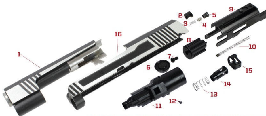
SP4-HXAA : slide, outer barrel & nozzle assembly
