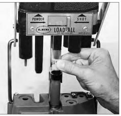
**STATION 3b** Raise handle, insert proper wad and lower the handle until it stops.
