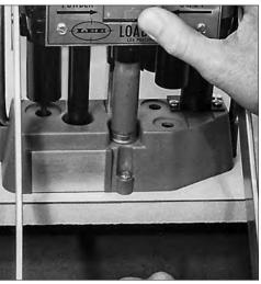
**STATION 3a** Lower the handle and slide charge bar to the right. This adds the powder.
