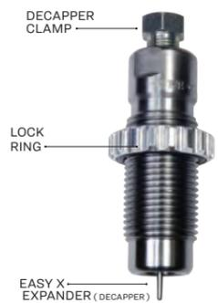
Screw the full length sizer in until it touches the shell holder. Then lower the ram and screw the die in 1/4 to 1/3 turn more. Raise the ram and tighten the lock ring finger tight.
