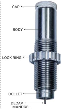
**ADJUSTMENT FOR LEE PRESSES** Screw sizing die in until it contacts the shell holder, plus one more turn (1 1/4 turns for Classic Series press owners).
