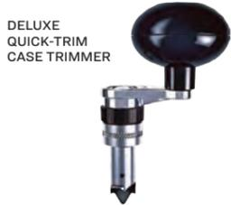
After a few loadings, cases tend to get longer. This could be dangerous if the case were so long that it would pinch the bullet in the end of the chamber. Pressure high enough to damage the gun could result. A convenient way to trim to the correct safe length is with the Lee Quick Trim Case Trimmer. Install the appropriate Quick Trim Die — and 5 quick turns of the crank will yield a perfectly trimmed and chamfered case. 90437 Deluxe Quick Trim
