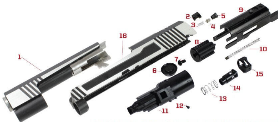
SP4-HXAA : slide, outer barrel & nozzle assembly
